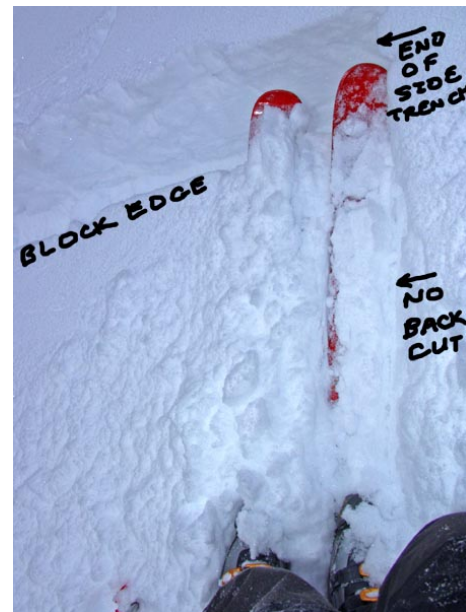
Fig. 2: Proper positioning at the top edge of the AK Block, with tips and tails over the side trenches, photo © Bill Glude.
